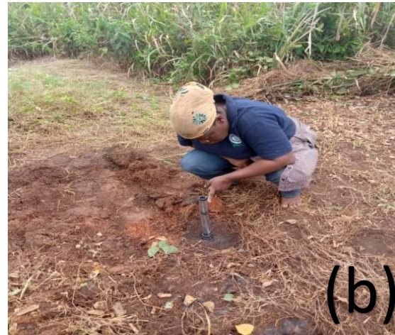
Plate 1: (a) Measurement of hydraulic conductivity on a bitumen deposit soil (LODA) (b) Measurement of hydraulic conductivity on a the control site (Legbogbo)
