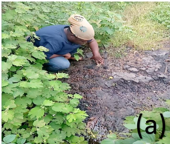
Plate 1: (a) Measurement of hydraulic conductivity on a bitumen deposit soil (LODA) (b) Measurement of hydraulic conductivity on a the control site (Legbogbo)
