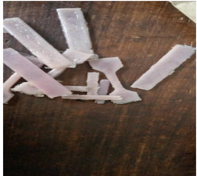
Figure 2. Specimen for tensile, hardness and impact test
