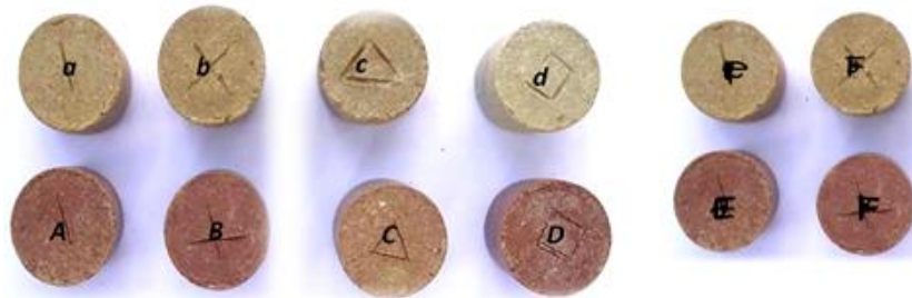
Fig. 10: Colour change of clay samples before (a,b,c,d,e,f) and after firing (A,B,C,D,E,F)
